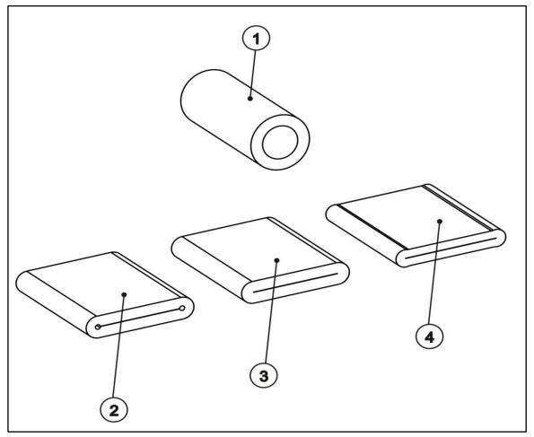
Fig. 3: Squeezing the hose
