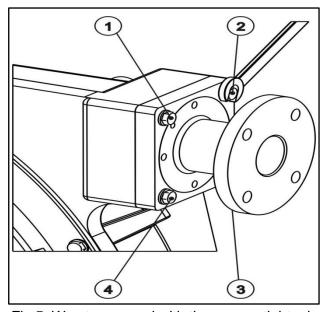
Fig.5: Way to proceed with the screws tightening
